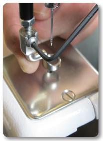
nut; center the foot with the needle; hold the foot in position; and firmly tighten the lock nut (Figure 9).
